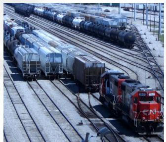
Flat switching yard: Switch crews classify cars into the proper tracks for the right outbound train.
