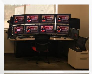
The **Rail Traffic Control Precision Dispatch System** (PDS) simulator replicates the functionality and operation of PDS features, allowing the **Rail Traffic Controller** (RTC) to practice various tasks such as lining signals, protecting movements, and responding to emergency situations.
