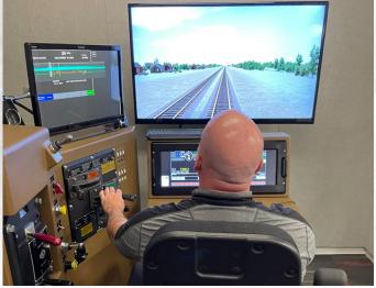
The Locomotive Engineer simulator replicates all controls of a real locomotive including: air brake handles, throttle handle, and all screens used to monitor train health and air pressure. Advanced safety features such as PTC and draft/buff force screens are also utilized to help trainees become proficient in the safe handling of their train.
