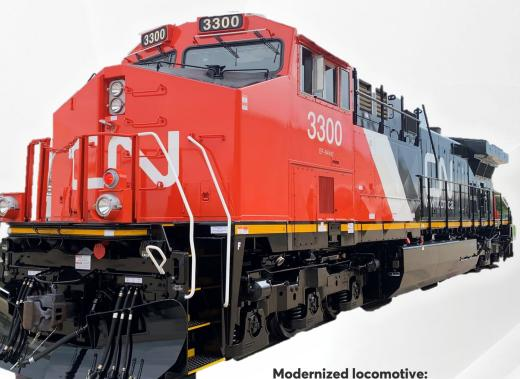
Transformed into a state-of-the-art 4,400HP AC unit.
