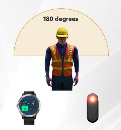
**Smart watch:** Provides yard employees with vibration and audible alerts for equipment moving in blind spot. **Rear-facing radar:** Worn on clothing / vest, equipped with flashing light for enhanced visibility.
