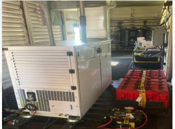
Inside of the box: Engine, Air Compressor, Battery, Air Brake and Electronics.
