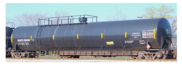
Pressure tank cars are used for the transportation of liquefied compressed gases (class 2 commodities) or the over-packaging of liquids. They have a tank test pressure ranging from 100 psi to 500 psi.
