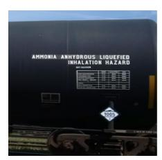
An example of a hazard warning on an Anhydrous Ammonia tank car
