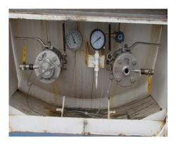
T50 (Spec 51) – pictured above. These tanks are designed for liquefied gases such as LPG or ammonia and have a capacity of around 5000 gallons. Their pressure relief device is mounted on the top and is recessed into the tank. The off-loading valves are located on the bottom corner inside a protective housing. A remote shut-off should be located on the right side of the tank, when facing the valve.
