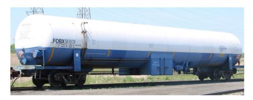
All of the tank's valves are in located in ground level cabinets that will be in the center of the tank car on either side or on opposite corners on either side of the tank car. Vent pipes must direct any product up and away from the cabinet or tank.
