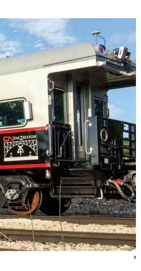
2 / The TEST car's autonomous track geometry system looks for track defects in Otto, Illinois (2015). 3 / CanaPux™ is a CN innovation (circa 2018).
