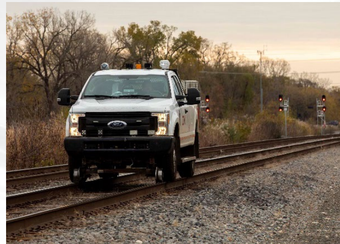
CN Hi-rail in the field: Revenue trains cannot occupy the same track while the hi-rail is performing a visual inspection.
