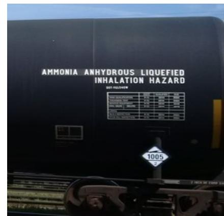
An example of a hazard warning on an Anhydrous Ammonia tank car
