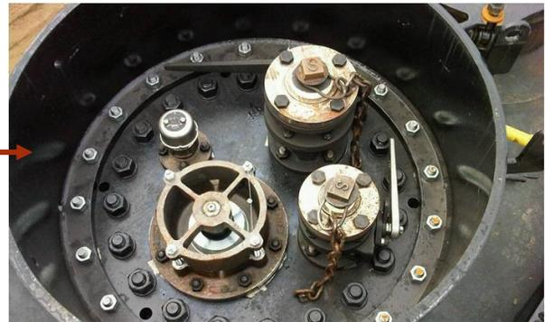
Legacy DOT-111 tank cars have combination housings. Combination housings are located on the top of these non-pressure tank cars, and house various valves and fittings.
