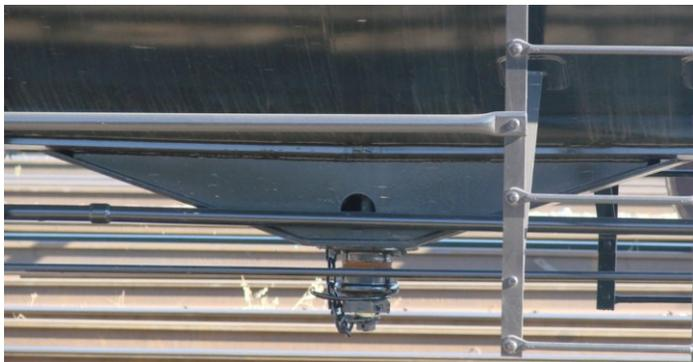
Bottom outlet valve on tank car, skid protection – external view
