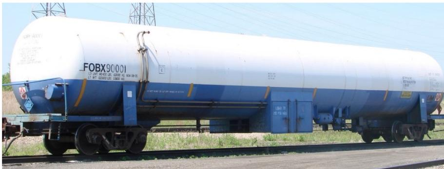
All of the tank's valves are located in ground level cabinets that will be in the center of the tank car on either side or on opposite corners on either side of the tank car. Vent pipes must direct any product up and away from the cabinet or tank.
