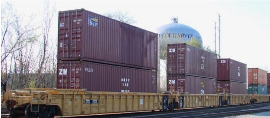
Some well cars may be in a "three-pack" or "five-pack" configuration. This means that although it may appear to be an individual well car, it is actually part of a larger articulated unit which shares sets of trucks. Each individual unit of a multi-unit well car configuration will have the same reporting mark (car number) followed by a letter to distinguish it, such as A through E.
