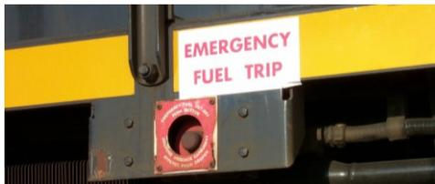
Each side of the frame of the locomotive, externally
