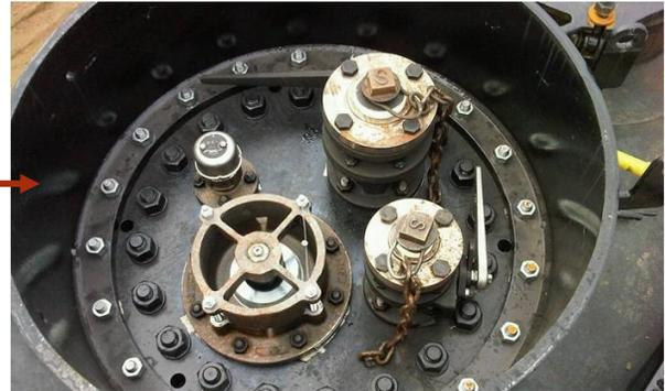
Legacy DOT-111 tank cars have combination housings. Combination housings are located on the top of these non-pressure tank cars, and house various valves and fittings.
