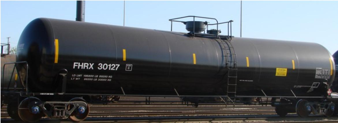
Non-pressure tank cars are also known as General Service, Low Pressure, or General Purpose tank cars. Acid Service tank cars are a subset of non-pressure cars. These will be referred to throughout this guide as non-pressure cars. Despite the name, these cars will have some pressure during transportation. The tank test pressure range is between 60 psi to 100 psi.
