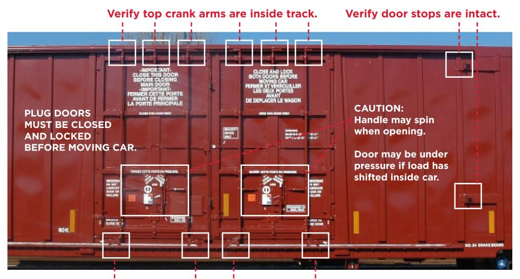
Verify rollers are on the track and pins are not broken.
