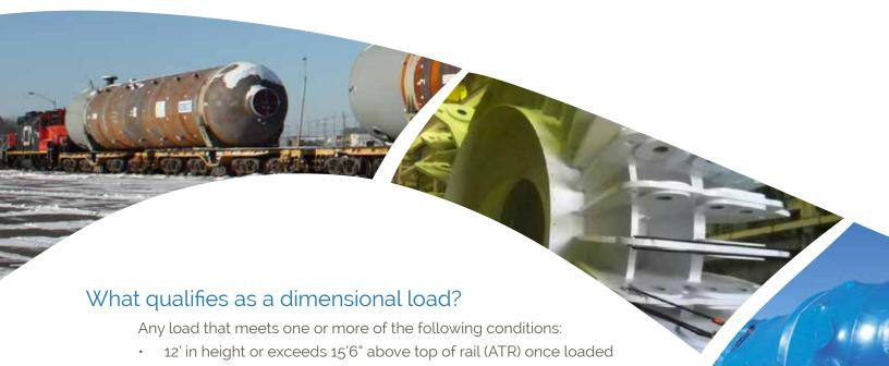
10'8" in width or exceeds length or width of the car deck and greater than plate "C"
