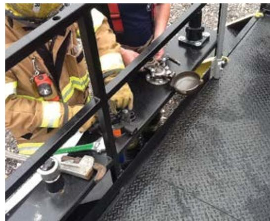
*Firefighters train to replace a tank car rupture disc on the CN dangerous goods training trailer.*
