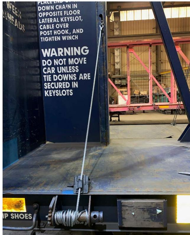
If the key slots and the hanger hook on the center beam upright post are damaged or missing, use securement option 3.
