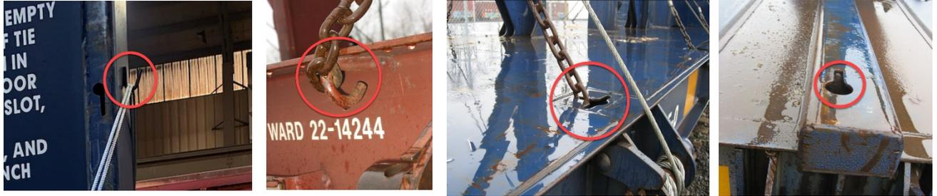
3. Tension cables until taut, do not over tension causing damage to car structure/components.
